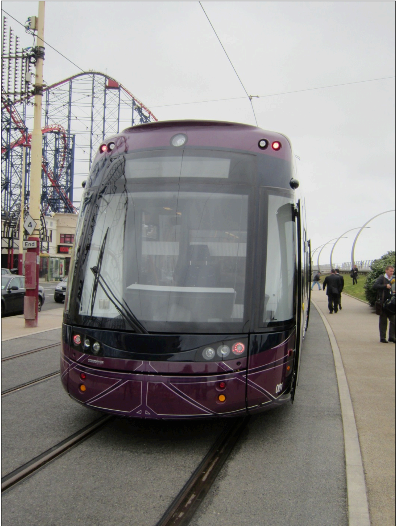
The cab end of the new tram opposite the Pleasure Park at Blackpool. The Flexity 2 design allows customers to choose the cab shape from a number of options. The tram is standing on refurbished track using the CDM Q(quiet) Track embedded rail system.
