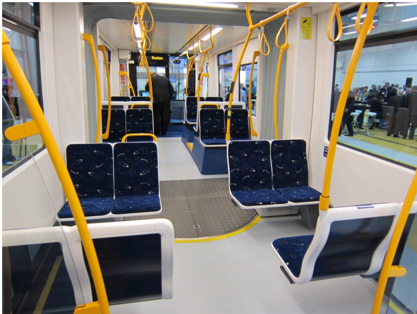
Interior of Flexity 2 tram looking towards the cab and showing the pleasant colour scheme. The seats nearest the camera are cantilevered off the car structure while those behind are mounted on wheel boxes.
