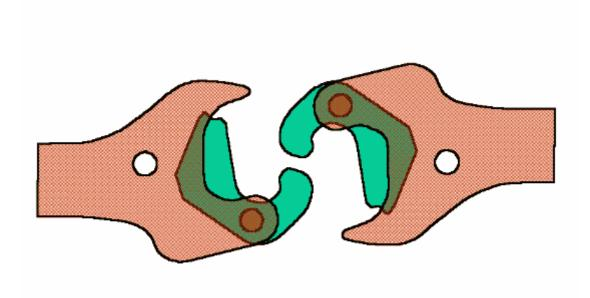
To couple two vehicles, the knuckles must be open. When the two vehicles are pushed together, the knuckles of the two couplers close on each other and are locked from behind by a vertical pin dropping a steel block into place behind a raised casting on the knuckle. To uncouple, one of the pins must be pulled up to release the block locking the knuckle. This is done by operating a lever or chain from the side of the vehicle.
